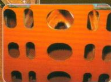
Triangular ribbed bed casting for improved support to guideways.
