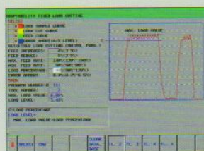
Adaptive cutting at constant loading
