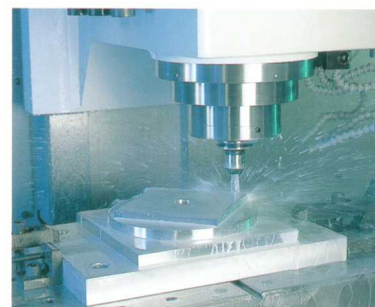
CTS (Coolants Thru. Spindle)
